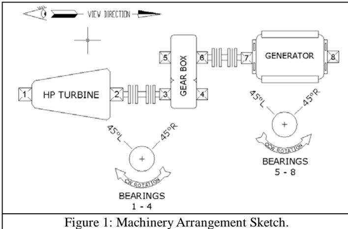
Figure 1: Machinery Arrangement Sketch.
