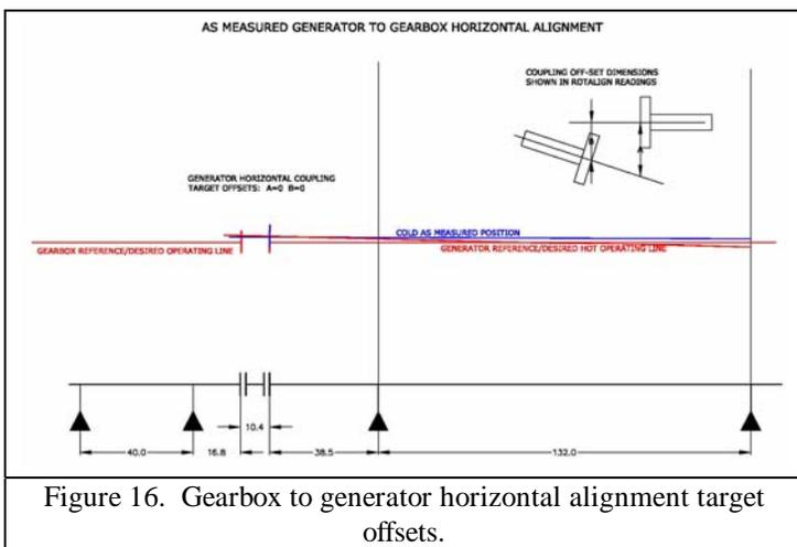
Figure 16. Gearbox to generator horizontal alignment target offsets.
