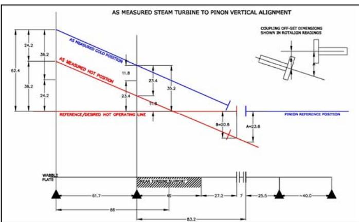
Figure 6: Hot and cold shaft relative alignment readings
