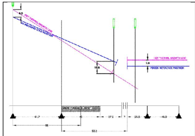
The blue lines represent the cold relative vertical shaft positions from the cold alignment check. The magenta lines represent the turbine and pinion shaft position changes based on the thermal growth measurements of a 9.5 mils rise at the turbine inlet end, a 15.8 mil decrease at the turbine exhaust end and a 7.6 mil rise of the pinion drive end bearing.
