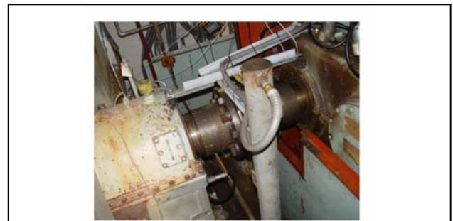
Photo 1: Growth probes at coupling area
