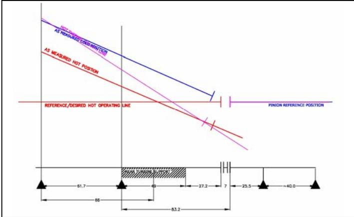
Figure 8: Comparison of cold/hot alignment readings and measured thermal growth readings. Magenta thermal growth lines translated so that pinion line lies on pinion reference line.
