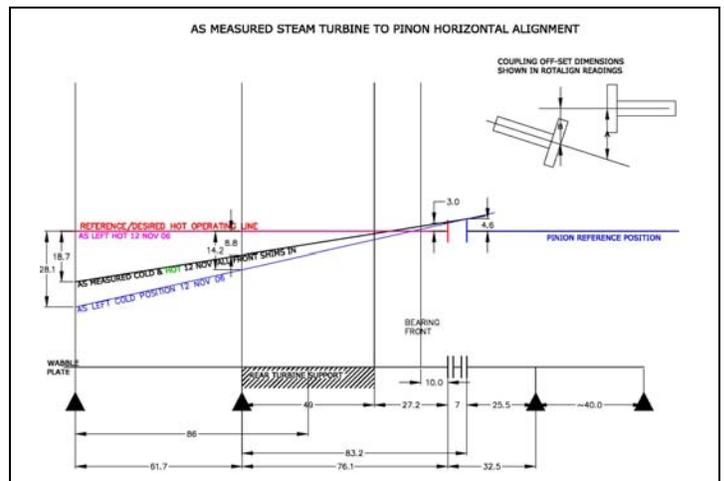
Figure 24. Horizontal cold alignment targets and as left cold/hot vertical alignment positions
