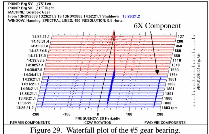
Figure 29. Waterfall plot of the #5 gear bearing.
