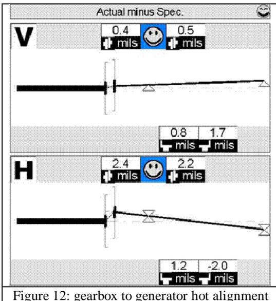
Figure 12: gearbox to generator hot alignment
