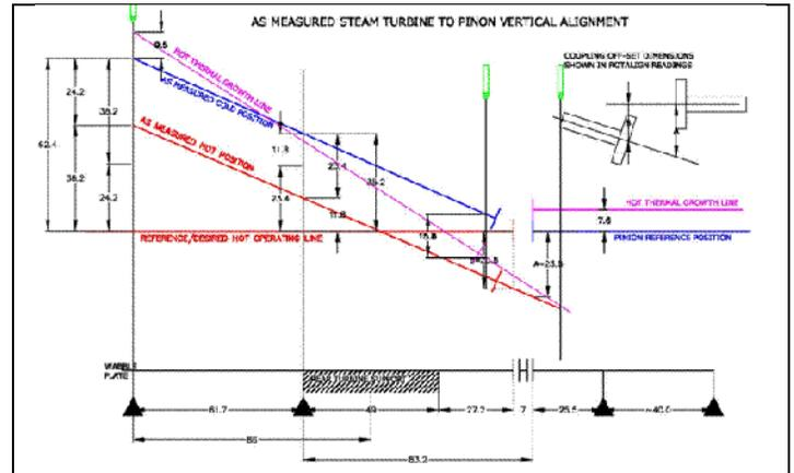
Figure 7: Hot and cold turbine/pinion alignment with thermal growth lines in magenta
