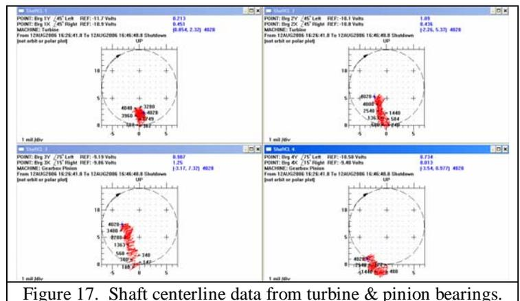
Figure 17. Shaft centerline data from turbine & pinion bearings.
