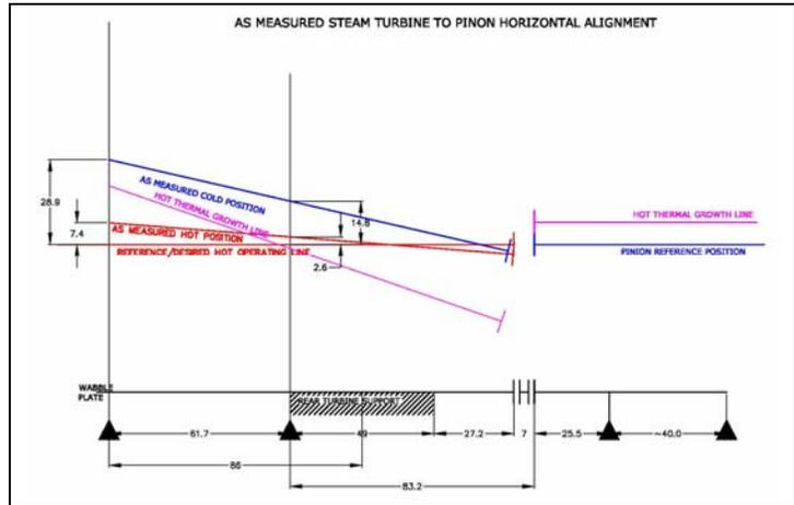
Figure 10: Horizontal cold and hot turbine to pinion alignment with hot thermal growth line.
