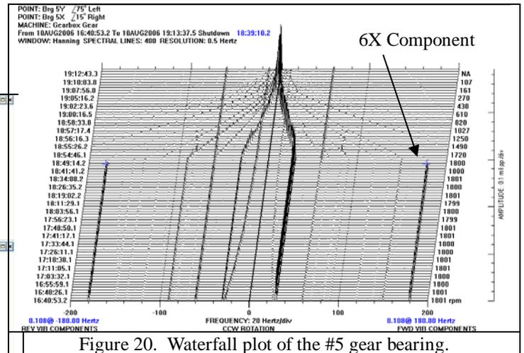
Figure 20. Waterfall plot of the #5 gear bearing.
