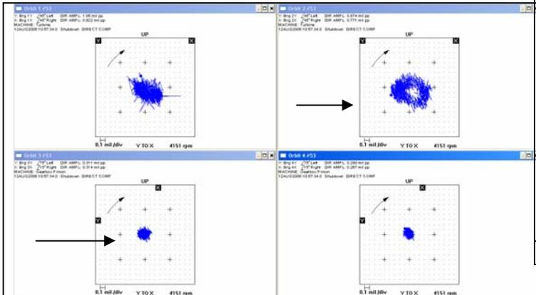
Figure 18: Direct (unfiltered) Orbits, Bearings 1,2,3 and 4
