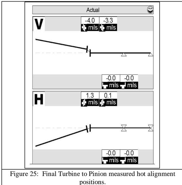
Figure 25: Final Turbine to Pinion measured hot alignment positions.
