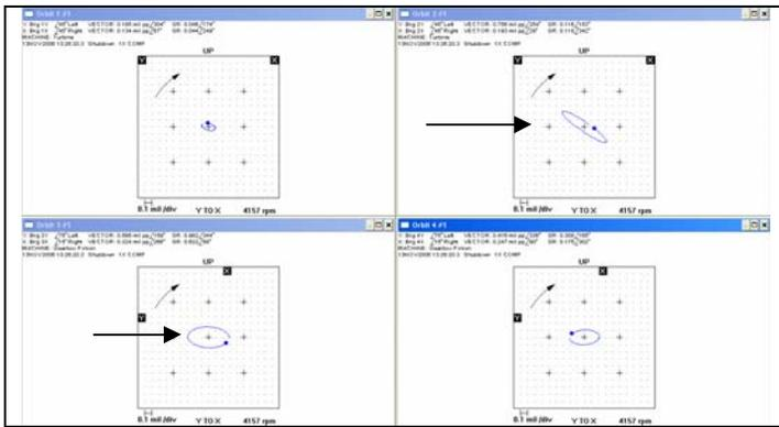
Figure 28: 1X Synchronous Filtered Orbits, Bearing 1,2,3 and 4
