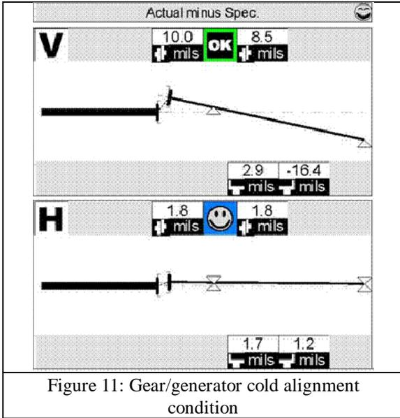
Figure 11: Gear/generator cold alignment condition
