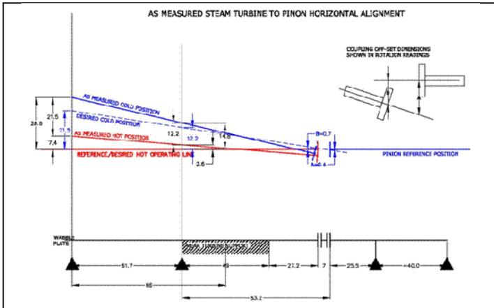
Figure 14. Desired horizontal cold alignment offsets between turbine & gearbox
