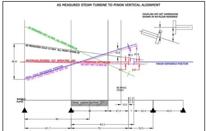
Figure 23. Vertical cold alignment targets and as left cold/hot vertical alignment positions.
