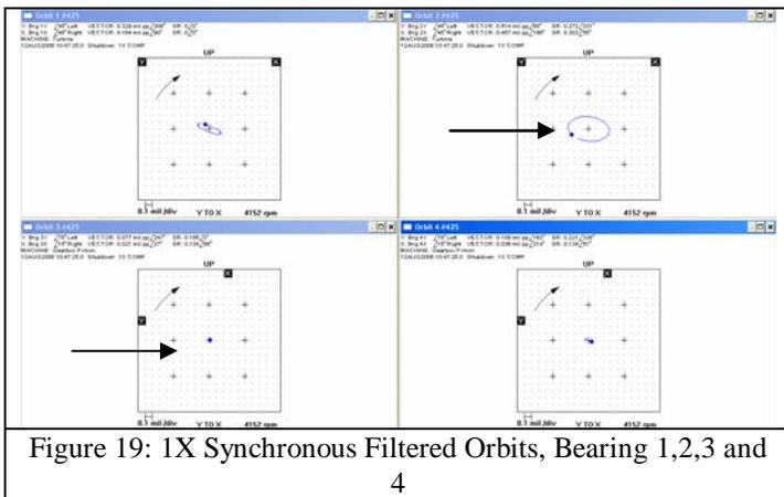
Figure 19: 1X Synchronous Filtered Orbits, Bearing 1,2,3 and 4
