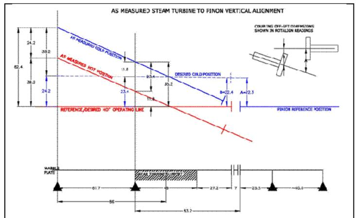
Figure 13. Desired vertical cold alignment offsets between turbine & gearbox.
