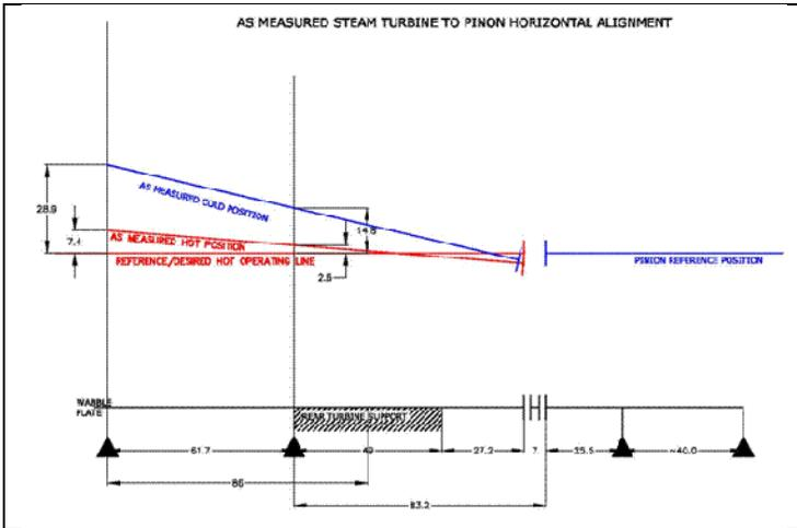
Figure 9: Horizontal cold and hot turbine to pinion alignment
