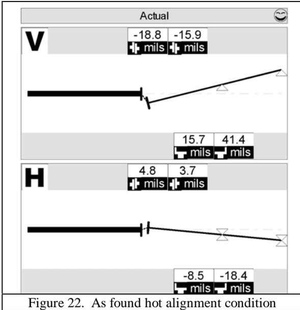
Figure 22. As found hot alignment condition
