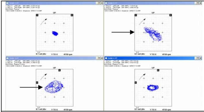
Figure 27: Direct (unfiltered) Orbits, Bearings 1,2,3 and 4
