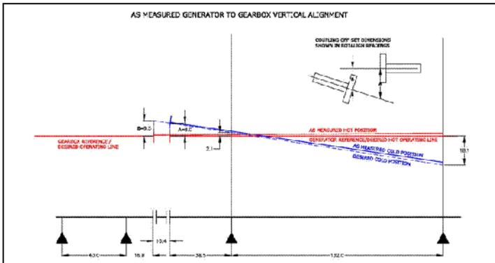
Figure 15. Gearbox to generator vertical alignment target offsets
