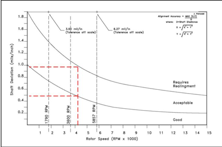
Figure 2: Coupling alignment tolerances.
