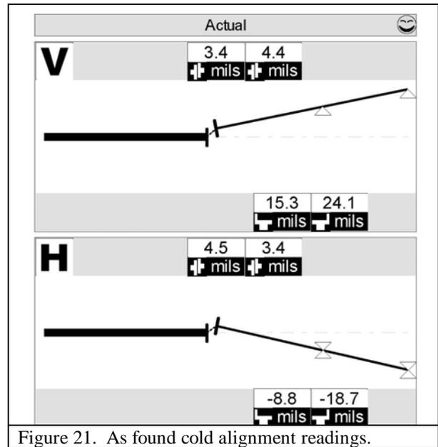
Figure 21. As found cold alignment readings.
