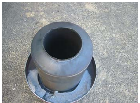
Photo 7: Disassembled silencer showing loss of packing material without physical damage to silencer
